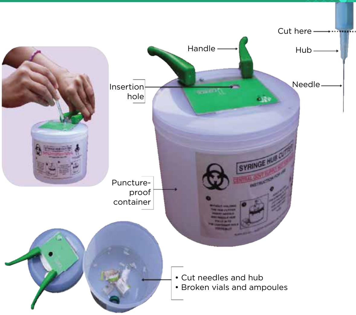
Figure 1: Correct use of a hub cutter. 9
