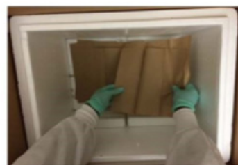
Place absorbent material
